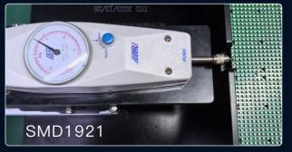
SMD1935 lamp bead withstands the thrust of 4.6kg
